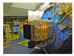
FIFI-LS Integral Field Spectrometer
